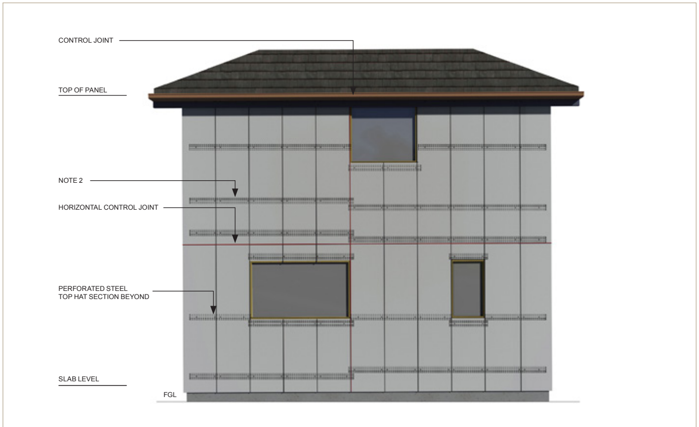
Detail 3.8 – Two storey construction – hip roof elevation
